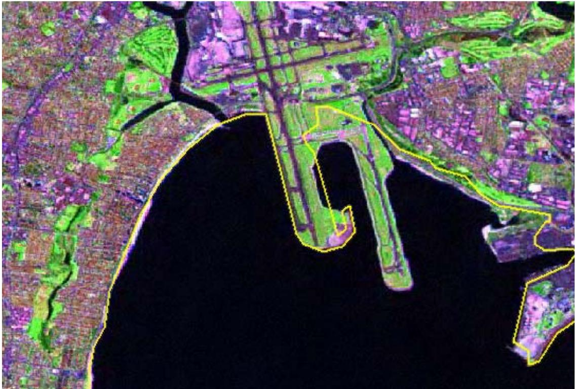
*An example showing the discrepancy between the GEODATA 100K coast and a more recent satellite image of Sydney airport. Note the changes to the first runway, the addition of the second runway and the build up of the area to the east of the airport.*
