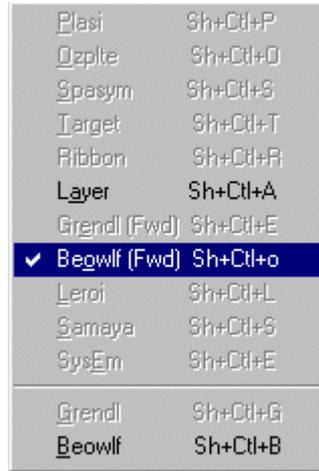
Select BEOWLF to operate in either the forward or inversion mode. If forward mode is requested, EM Vision will display a dialog to report that this mode has been selected. If BEOWLF inversion mode is chosen a dialog to control the number of iterations and noise-to-signal ratio is displayed.
